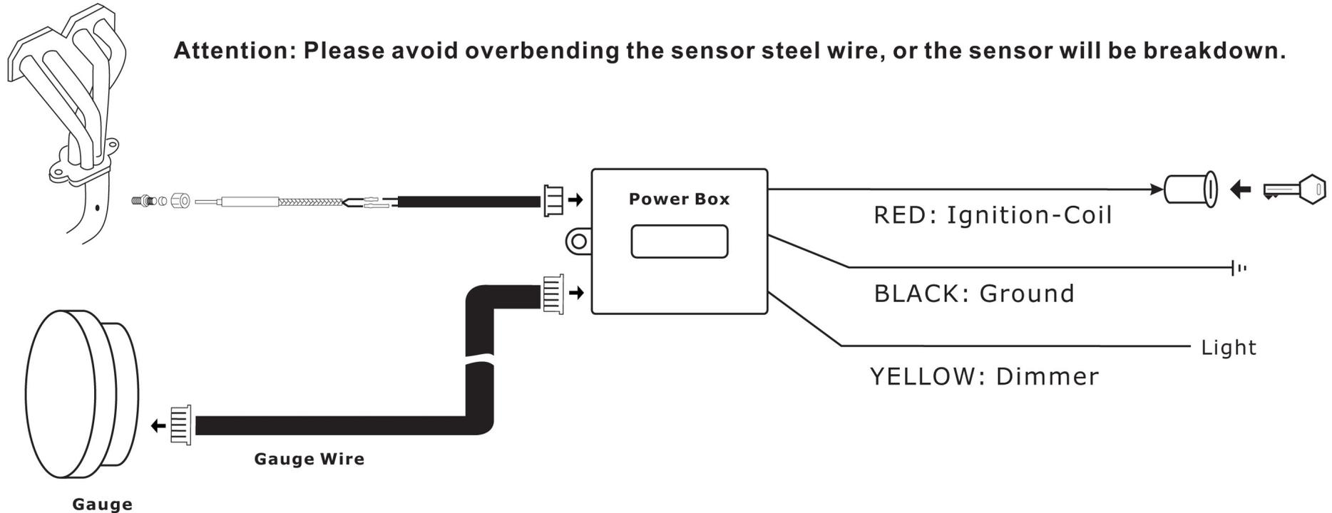
To avoid damage, please ensure the RED wire is attached to the ignition switch that connected to Coil.
